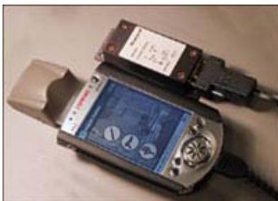
Fig. 7: The PDA with the compass and GPS attached
